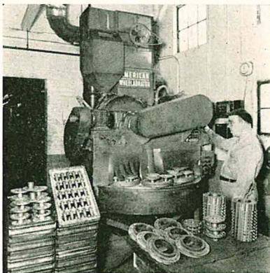
The Wheelabrator Swing Table which handles 80% of all Airblast Room jobs and is capable of cleaning a wide range of large and small pieces where the daily production does not warrant the cleaning of several different types of equipment.
