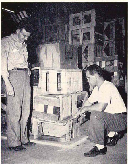
Willard Flowers points out to Stanley Hes improper stacking of material — motors in this instance. This has resulted in the damage of a crate, and the possibility of a man being scratched by the protruding slat.
